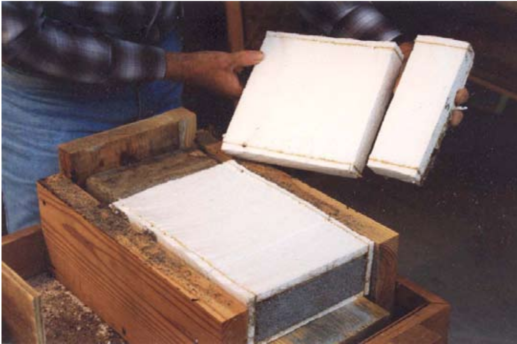
#64 TEST FIXTURE - Close-up shows no termite damage.
