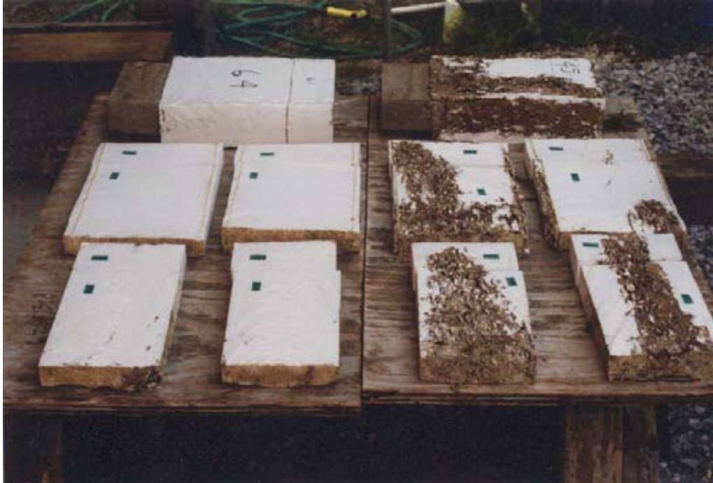
#64 TEST FIXTURE - Perform Guard EPS and R-Control Do-All-Ply.
