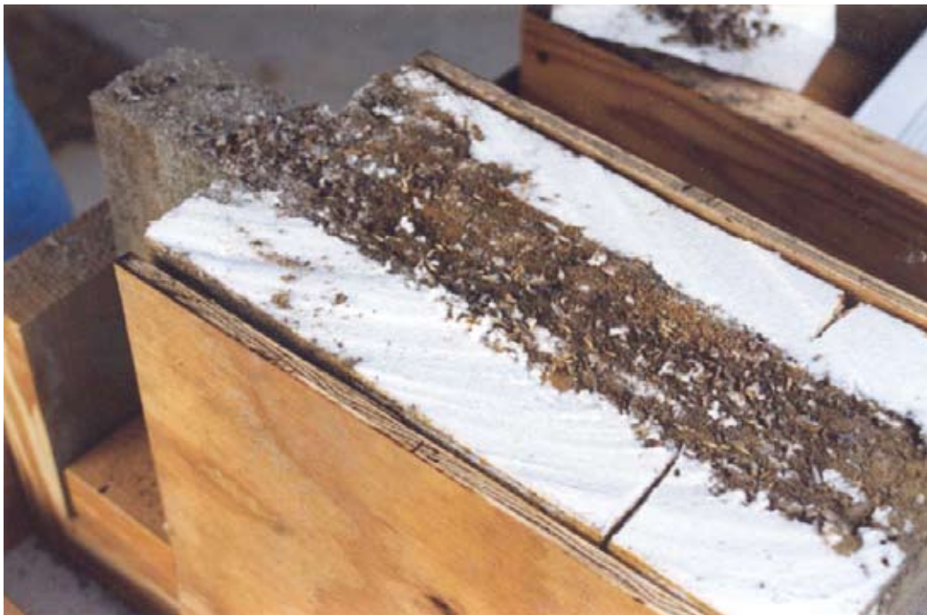
#45 TEST FIXTURE - Close-up shows active termites.
