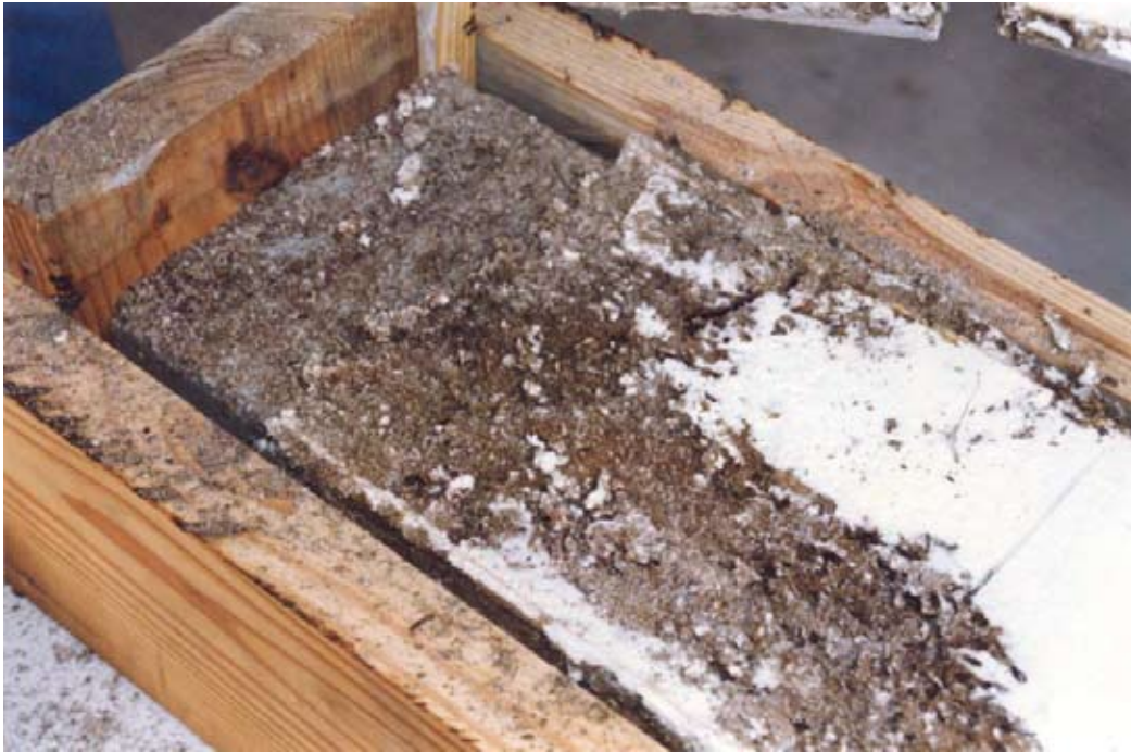
#45 TEST FIXTURE - Close-up shows extensive termite damage.
