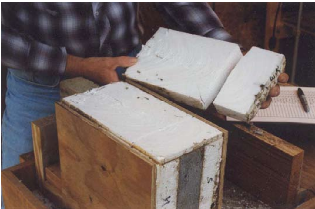
#64 TEST FIXTURE - Close-up shows slight termite damage.
